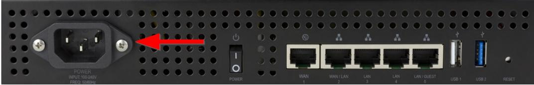
3. Connect an ethernet cable from your computer to any of the LAN ports on the router.
